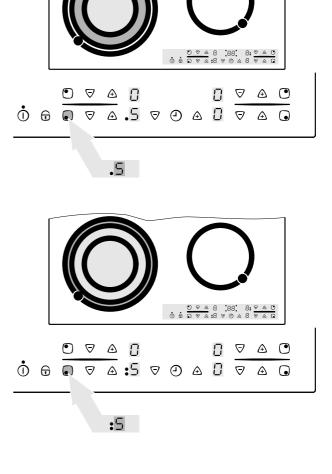
4. In order to switch off the outer heating ring,
